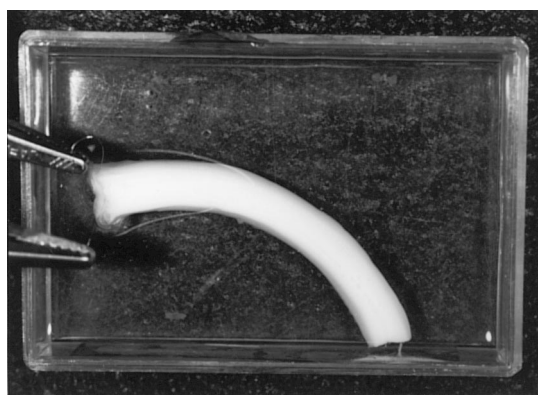
Figure 14 Bending of the PVA–PAA hydrogel rod.
